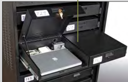
#050-00747 Secure Laptop Drawer (can accept laptops up to 14.75" x 12" x 3" high). Secure Laptop Drawers come complete with a 2-outlet power bar and has (2) private chambers with lockable lids. Note: Each lid is keyed differently to all other lids in the cabinet or cabinets unless specified. Master Keys available. Space required: 6"
